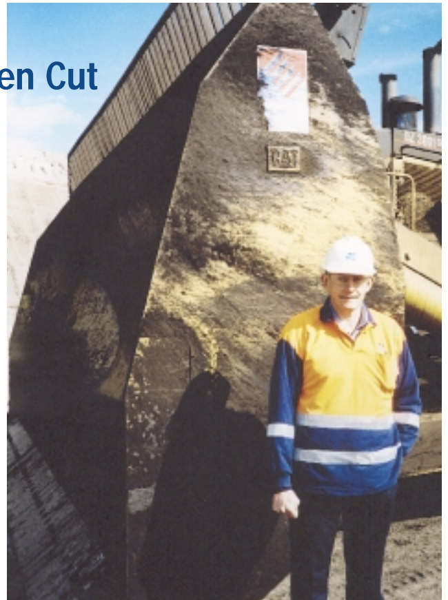
Bill Otto, Electrical Superintendent for the Roche Thiess Linfox Joint Venture, is dwarfed by the massive blade of a D11 dozer. These machines push 80 tonnes at a time to the Feeder/Breakers.
